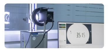
With the new devices, we are now able to calibrate all dial gauges, limit plug gauges, thread plug gauges and setting rings ourselves in the factory and make them available again within just 48 hours.
