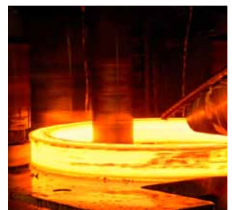
Our partner firm ROTEK in the USA even possesses a roller mill for producing race rings for large antifriction bearings.
