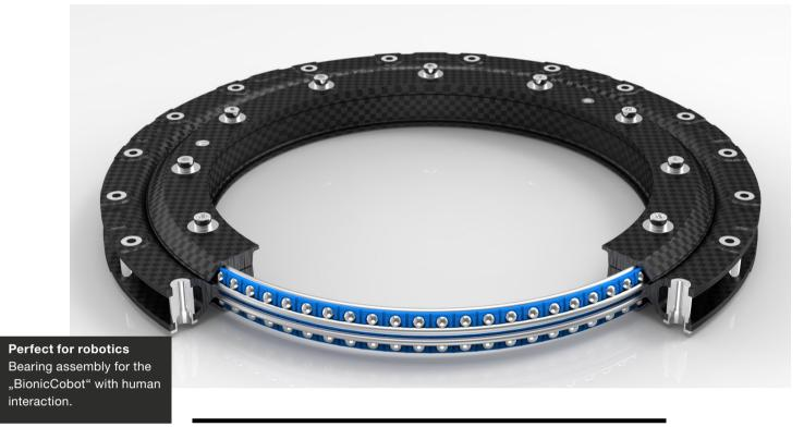
Lightweight robots are increasingly used as service and mobile robots. The mass of such robots rarely exceeds 10 kg with a typical nominal load of 3 kg. They consist of light CFRP materials with good stiffness and low mass. Space-saving bearings are used for the motion axes, which have a high stiffness, low weight and a small installation space.
