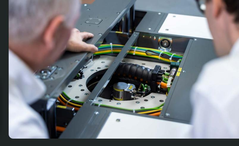
The heart of the drive The large center clearance of the Franke bearing assembly creates space for cables and components
