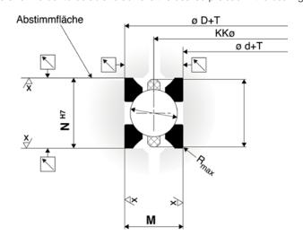
The wire bed has no radii which accommodate the race. However, care must be taken in the design that the tool radii are not greater than 0.2 mm.
